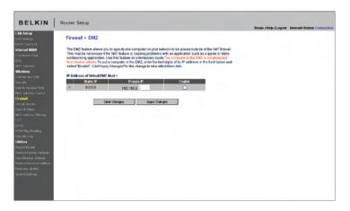
To put a computer in the DMZ, enter the last digits of its IP address in the IP field and select "Enable". Click "Apply Changes" for the change to take effect. If you are using multiple static WAN IP addresses, it is possible to select which WAN IP address the DMZ host will be directed to. Type in the WAN IP address you wish the DMZ host to direct to, enter the last two digits of the IP address of the DMZ host computer, select "Enable" and click "Apply Changes".
